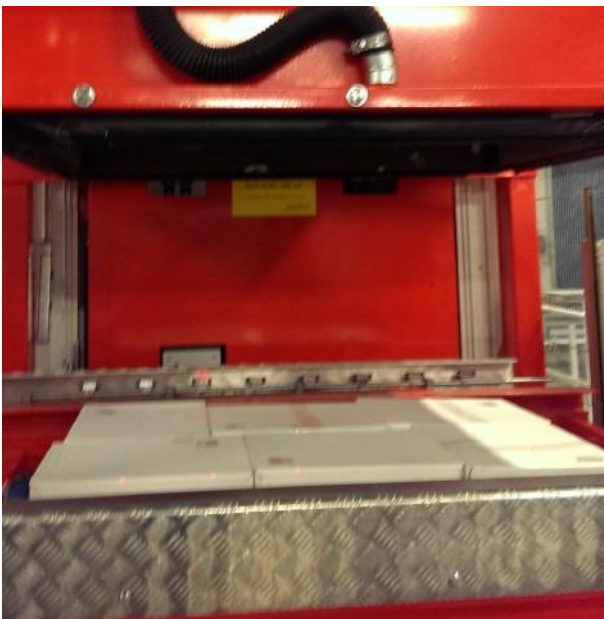
An automatic depalletiser ready to lift a layer off the pallet.
